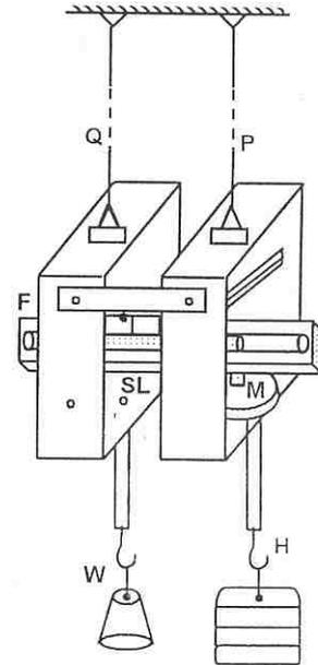
The load on the hanger is reduced in the same steps and spirit level is restored to horizontal position. The mean of these two observations gives the true increase in length of the wire corresponding to the given value of load.
